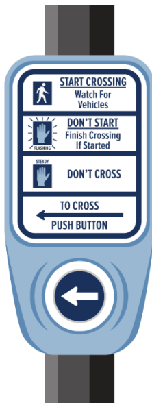
Figure C7 – Pedestrian Signal Push Button
