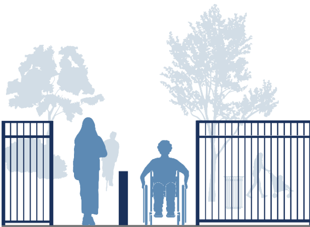
Figure D16 – Clear Width Between Bollards
